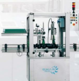
detail distributoru a tepelné hlavy + distributor kapslí s tepelnou hlavou
